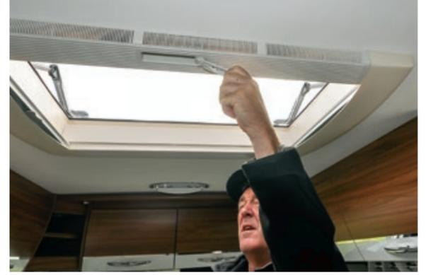
The 820mm x 520 panoramic sunroof opens with a winder and is on stays, what a great idea instead of push open and pull close - no blowing up in the wind with this model
